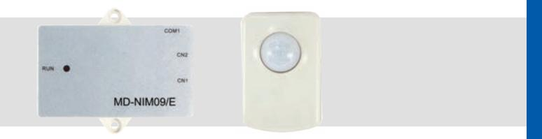
Thanks to the infrared sensors the device detects motion and this enables control of the indoor unit. If the room remains unoccupied for 30 or 60 minutes, the air-conditioner will stop operating and resume automatically after detecting motion.
